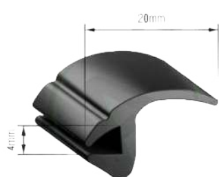
PRB104 EPDM 20 mm With Groove - Glue in Windcreens Profile
